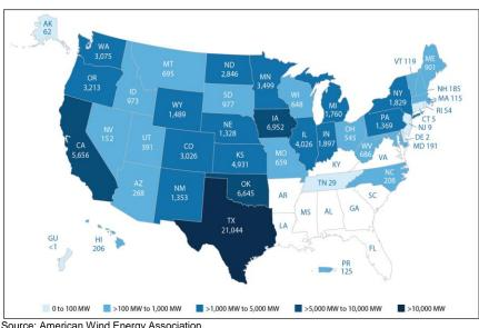
U.S. Wind Capacity, Q1 2017 (MW)
