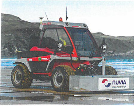
The Metrac vehicle and Groundhog system in use at Strathy beach near Dounreay, UK (Credit: DSRL, NDA and Nuvia)
